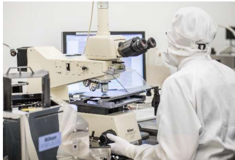
Inline-quality-management of processed Wafer ©Fraunhofer IPMS – Fotograf: Brandt
